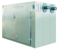
and automatic temperature control system. The whole circulating system is fully sealed, it makes the hot efficiency increased (from traditional oven's 3%-7% to current 35%-45%), the highest heat efficiency can be reached 70%. The success of this oven's invention makes Chinese hot air circulating oven meet the advanced level in world, it saves energy and raises the economic benefit. In 1990, Chinese medical management bureau issued the industry standards as RXH.
